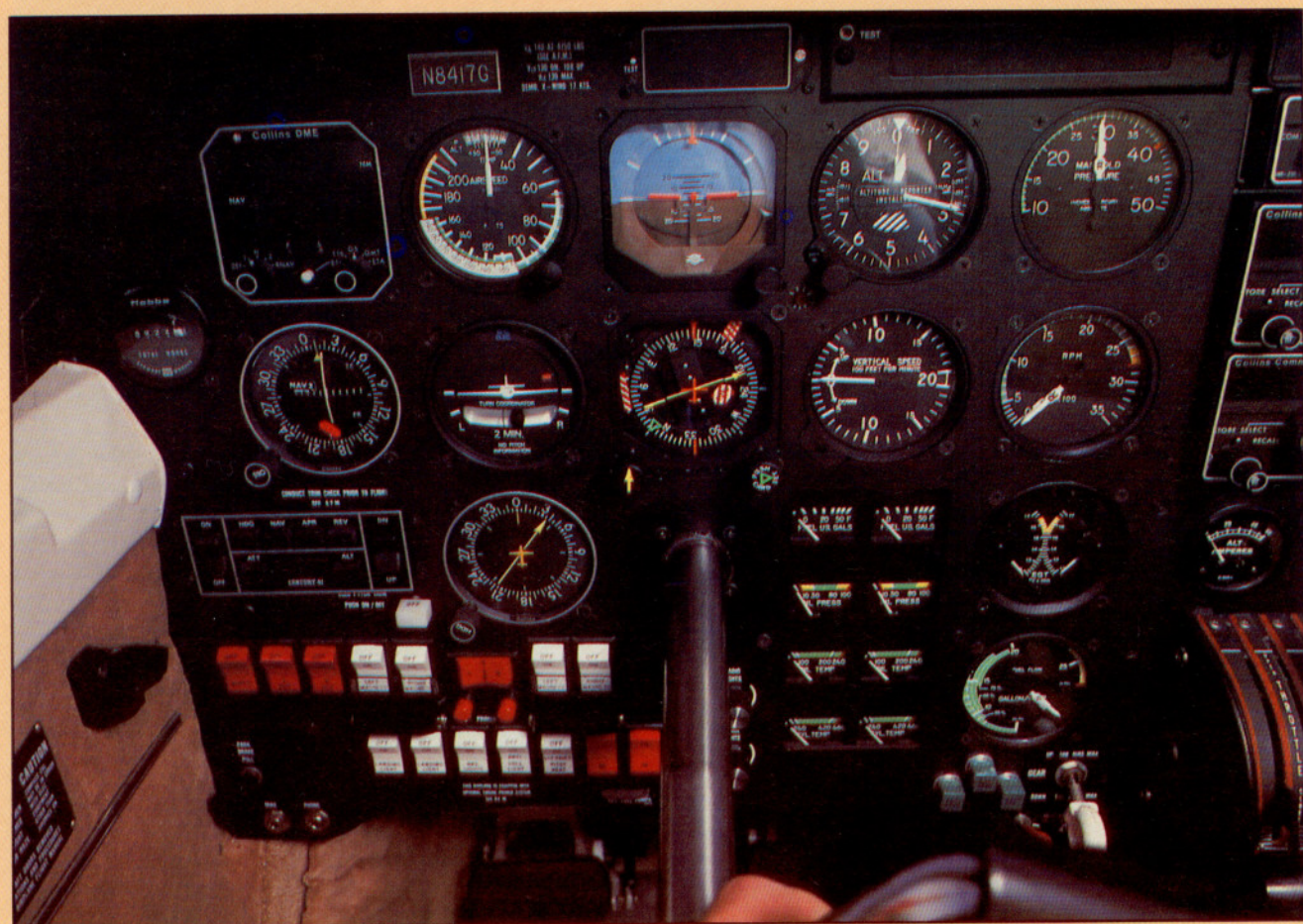
Gone are the windshield post and the plastic panel. The new metal panel has an improved arrangement of instruments and good lighting.
